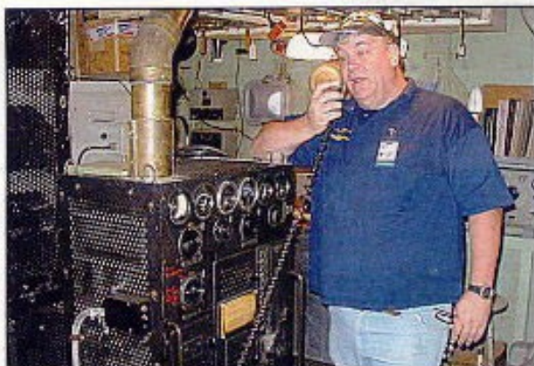
This is Bob, W1QWT, on 3885 kHz, 100 watts AM, with original ship equipment, a TCK-4 transmitter.
